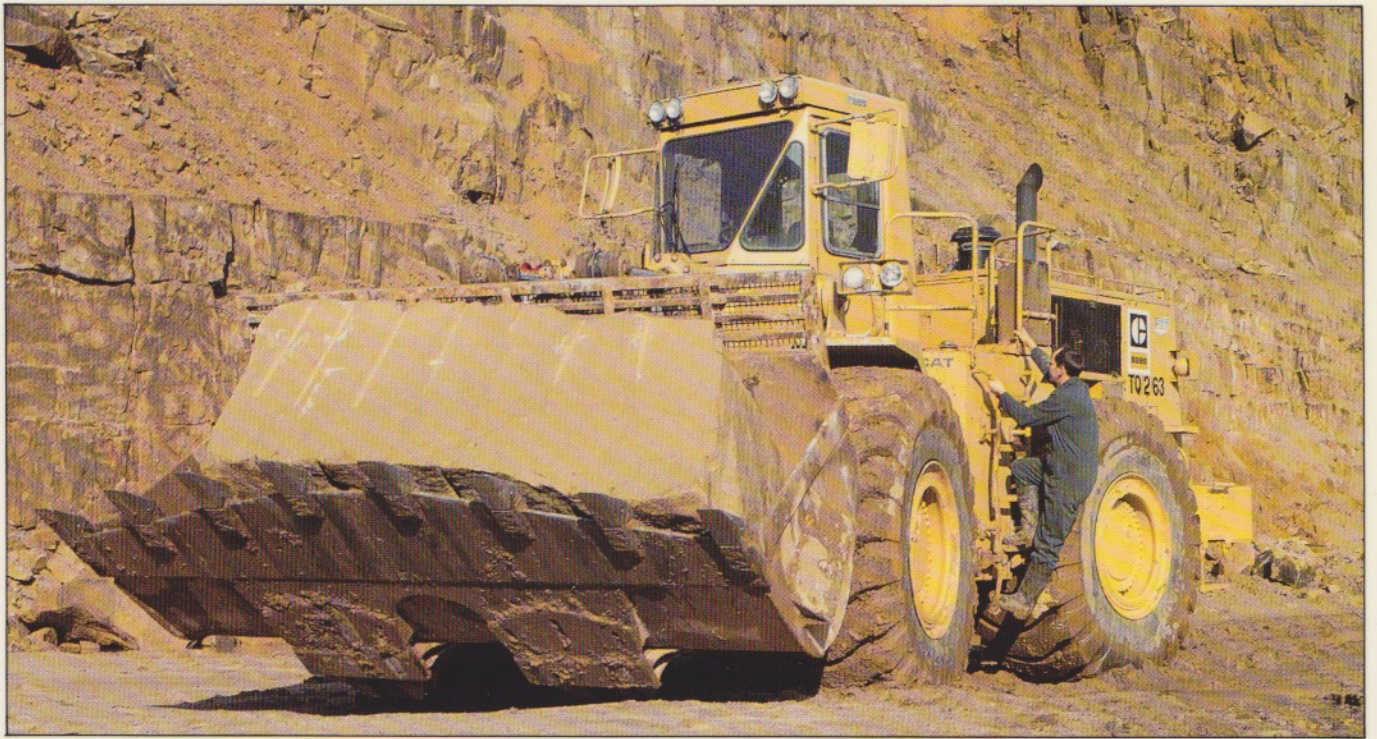
Cat 988B transporting large blocks of stone from the quarry face to the saw sheds
